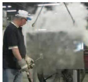
*Electro-Steam Generator's model LB 40-60 cleaner's design consists of a high-pressure chamber filled with water that is heated by one or more submerged resistance-type electric heating elements. Automatic controls maintain a pre-set operating pressure and water level.*
